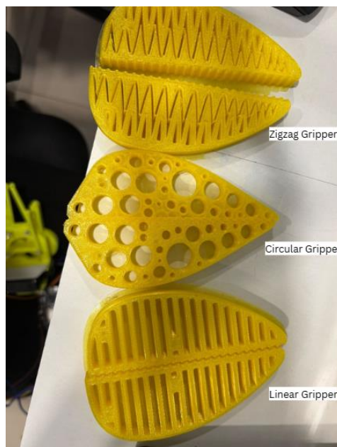
Figure 1. TPU Printed Grippers with Different Internal Geometries
